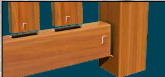
Showing how notched rails fit into routed posts and notched pickets fit into routed rails for assembly.
